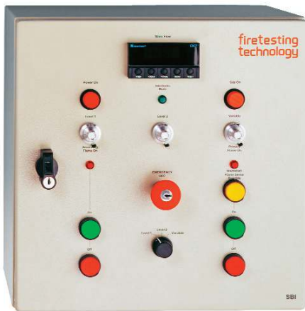
Gas Control Box
